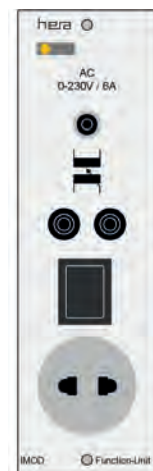
MP Module with jacks and universal socket for floating voltage (with selector switch)
