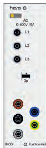
MP Module with jacks (non floating)
