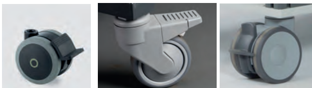
Standard 75mm max. load: 150kg height: 130mm Heavy Duty: 100/125mm max. load: 300kg height: 190/210mm Design 100mm max. load: 300kg height: 120mm
