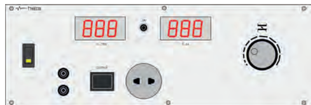
Variable AC source FLOATING (1,5EP)
