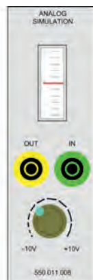
550.011.008 Analogue +/- 10V In- and Output with Counter and Simulation Potentiometer
