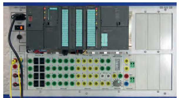
Exemplary Set-Up of PLC Panel 1 (PLC and Mudules have to be ordered seperately)
