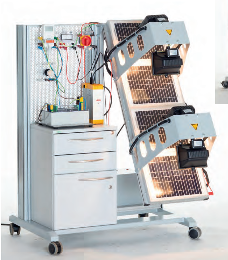
PROFI Photovoltaics Mobile, with tilt adjustment, foldable for compact storage, measuring units hooked in installation wall
