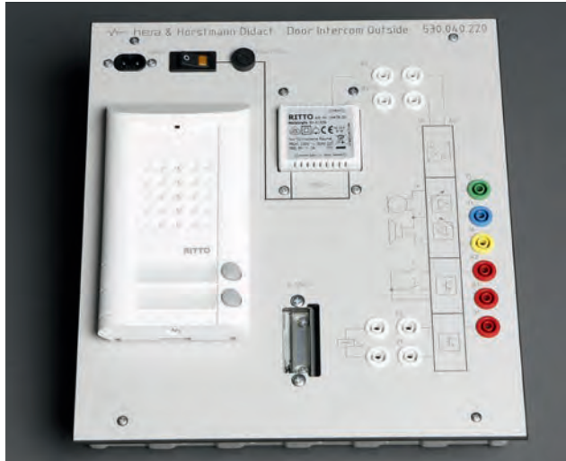
Door Intercom Point outside 530.040.220
