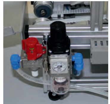
Maintenance Unit for Compressed Air
