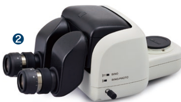
2 P2-TERG50 Trinocular Tilting Tube (eyepiece: port 100:0/50:50)
