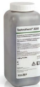
Technotherm 3000 with graphite filler is the electrically conductive product of the Technotherm range. Technotherm 3000 is used where high electrical conductivity is indispensable (e.g. for scanning electron microscopy). Voltage losses are almost excluded (less than 0.5%) when examining samples in the SEM with Technotherm 3000.
