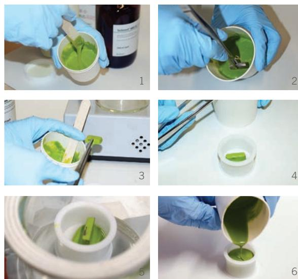
1-Mix Technovit 4002 IQ. 2-Dip in porous specimen. 3-Remove specimen. 4-Position in mounting mould. 5-Draw vacuum in Vacuum-Set. 6-Fully fill specimen with Technovit 4002 IQ.
