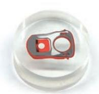
Technovit® 2000 LC is ideal for target preparations in microelectronics and mounting of polymers.
