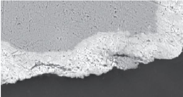
The system can be used for all types of material, however especially for porous materials, e.g. porous spray coatings or corrosion layers which are preferably embedded under vacuum. The vacuum impregnation effects the penetration of the mounting medium into even the finest cavities and stabilises porous materials optimally for further processing.
