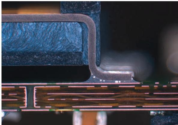
Gap-free mounting of an SMD plug from the electronics of a mobile phone in the dark field
