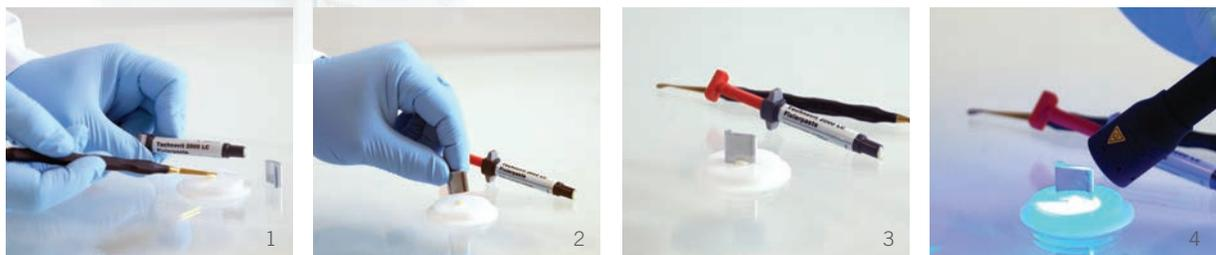
Fig. 1: Place Technovit fixing paste (page 15) on the bottom of the mounting mould. Fig. 2+3: Position specimen. Fig. 4: Cure fixing paste with the Technovit Blue LED. Embed specimen as usual.
