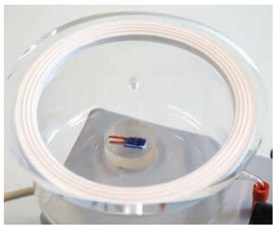
Draw vacuum in the Vacuum-Set, Technovit 2220 penetrates into any existing gaps
