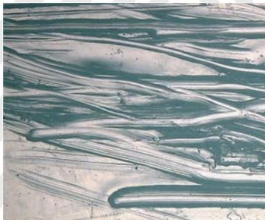
Identification of microcracks with ambulatory metallography
