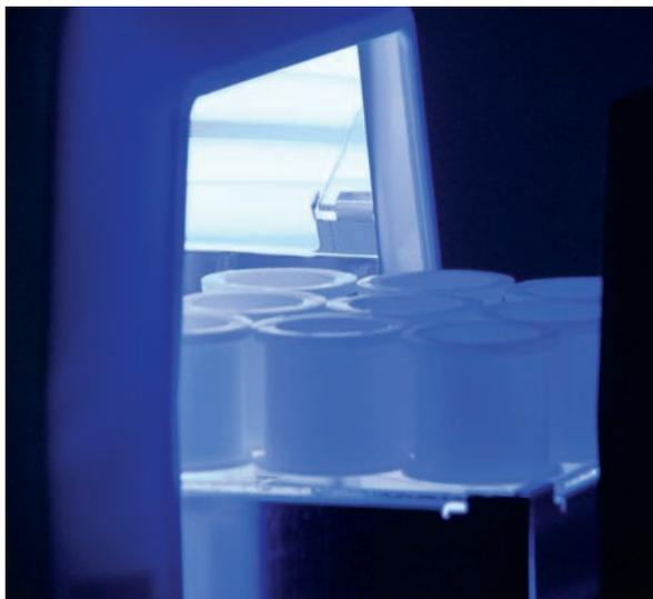
Homogenously illuminated specimen chamber with room for up to 9 specimens. Autostart and Timer
