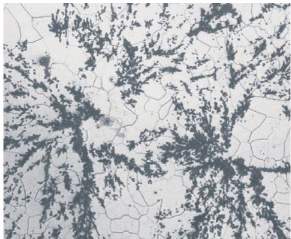
Original and impression of a mould. Ferritic grey cast iron with rosette-shaped arrangement of the graphite. Etched with 3% nitric acid.
