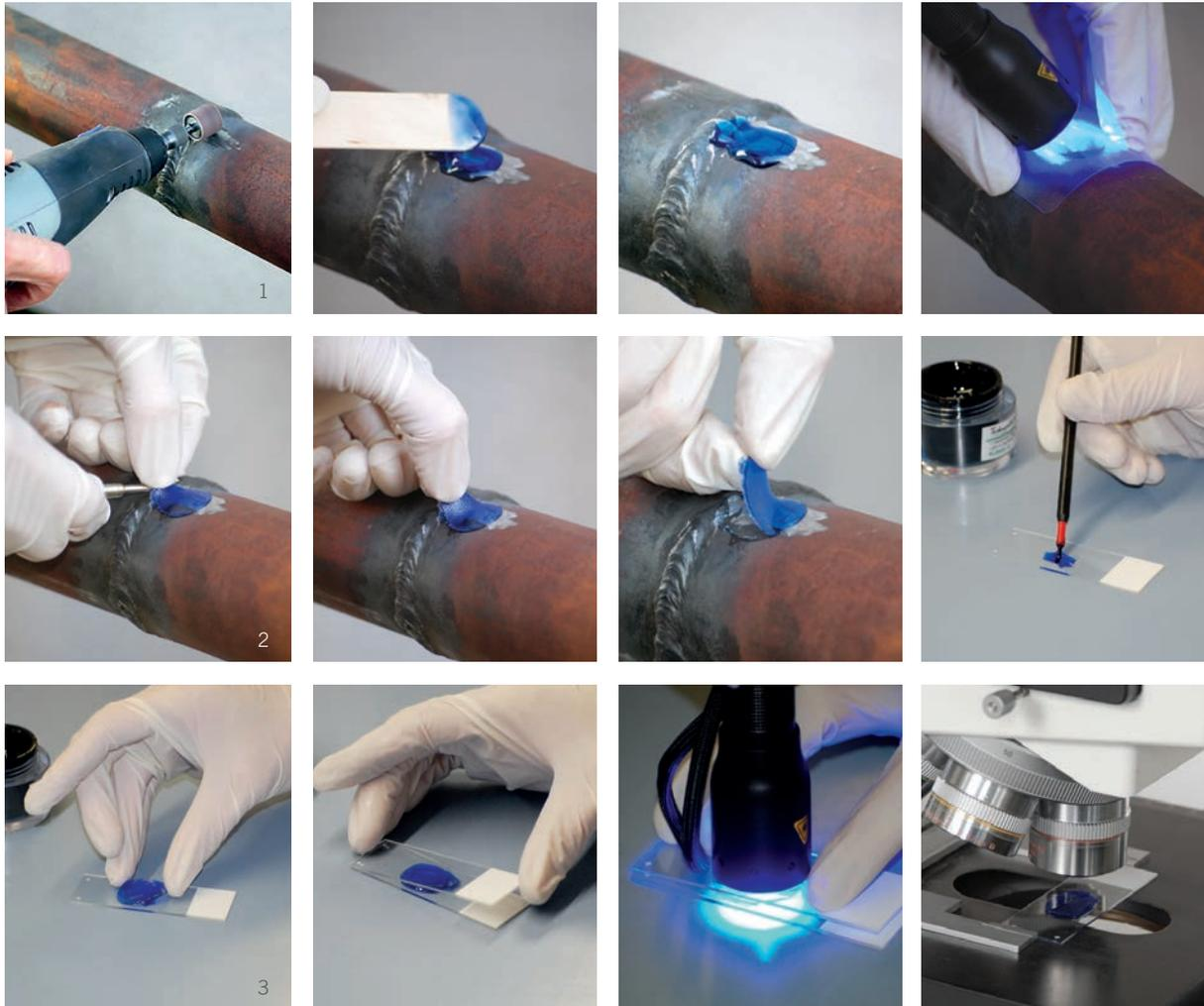
1. Grind slightly, polish, etch, apply Technovit 2220, spread thinly with a film, cover and polymerize.
