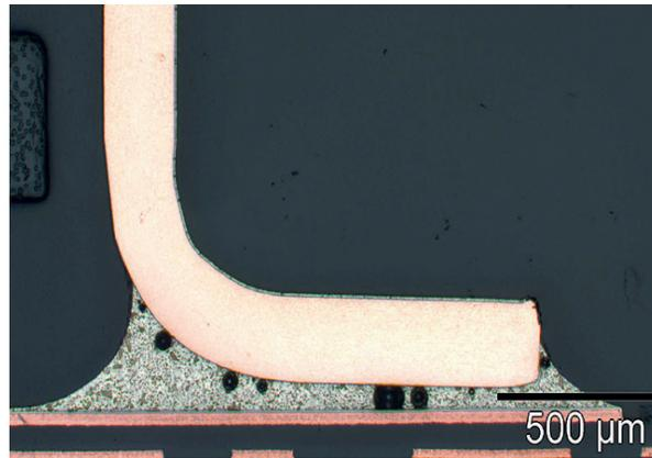
Enlarged detail of the CU contact pin of the component in the bright field
